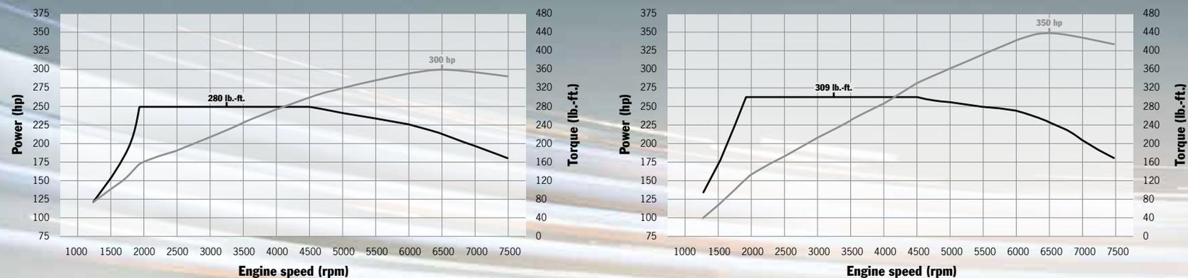
718 Boxster and 718 Cayman: 300 hp at 6500 rpm, 280 lb.-ft. between 1950 and 4500 rpm
